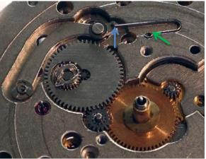
Put a little D5 where you see the 3 blue arrows. First put the hour wheel over Cannon pinion, then put the date
