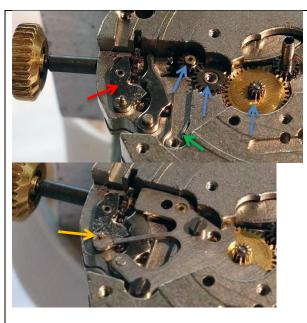
260: Minute wheel 440: clutch lever spring
