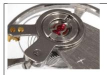
Add just a tiny drop of Moebius 9010 through the center of the bezel shaft and pierced jewel. Do not touch the shaft with oil.
