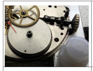
13 – Put the barrel with main spring and winding stem back in position.
