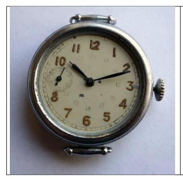
22 – Turn the movement, put the centre wheel in position, add the dial (tightened with 3 little screws on the side of the movement). Add the seconds, hour and minute hand.
